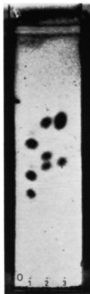
FIG. 7. TLC of keto bile acids with solvent system S9. Compounds are enumerated in their order from the starting line. Me = methyl ester; Et = ethyl ester. 0 = origin. Position 1 : 3 \alpha ,7,12-diketo; 3 \alpha ,7 \alpha ,12-keto; 3 \alpha ,12 \alpha -7-keto; 7 \alpha ,12 \alpha ,3-keto. 2 : Me-3 \alpha ,12 \alpha -7-keto; Et-3 \alpha ,12 \alpha ,7-keto; 3 \alpha ,12 \beta . 3 : Me-3 \alpha ,12 \alpha ,7-keto; 3 \alpha ,12 \alpha ; 3 \beta 12 \alpha .
